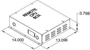
This must be used in conjunction with remote cpu ER104-XXX Recommended clearance for display with lens is 1.50 inch.
