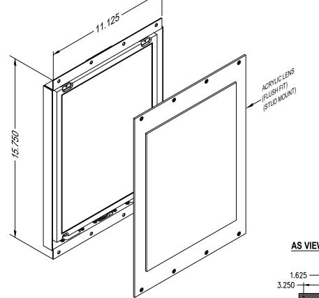
Main Screen is 3 Inches Deep Auxiliary Screen is 2-1/4 Deep 3-1/2 Inch Box Depth Recomended
