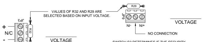
THE TIMER INPUT ALLOWS THE USER TO CONNECT AN OPTIONAL EVENT TIMER TO THE SECURITY SYSTEM. THE TIMER IS USED TO SET A SCHEDULE FOR FREE AND SECURE ACCESS TIMES FOR ANY OR ALL OF THE FLOORS ON A 7-DAY OR 365-DAY SCHEDULE. DIP SWITCH 3 DETERMINES IF THE SYSTEM USES AN ACTIVE HIGH (VOLTAGE APPLIED) OR ACTIVE LOW (VOLTAGE REMOVED) SIGNAL TO PROVIDE FREE ACCESS TO THE SYSTEM. SEE THE USER'S MANUAL FOR MORE INFORMATION.
