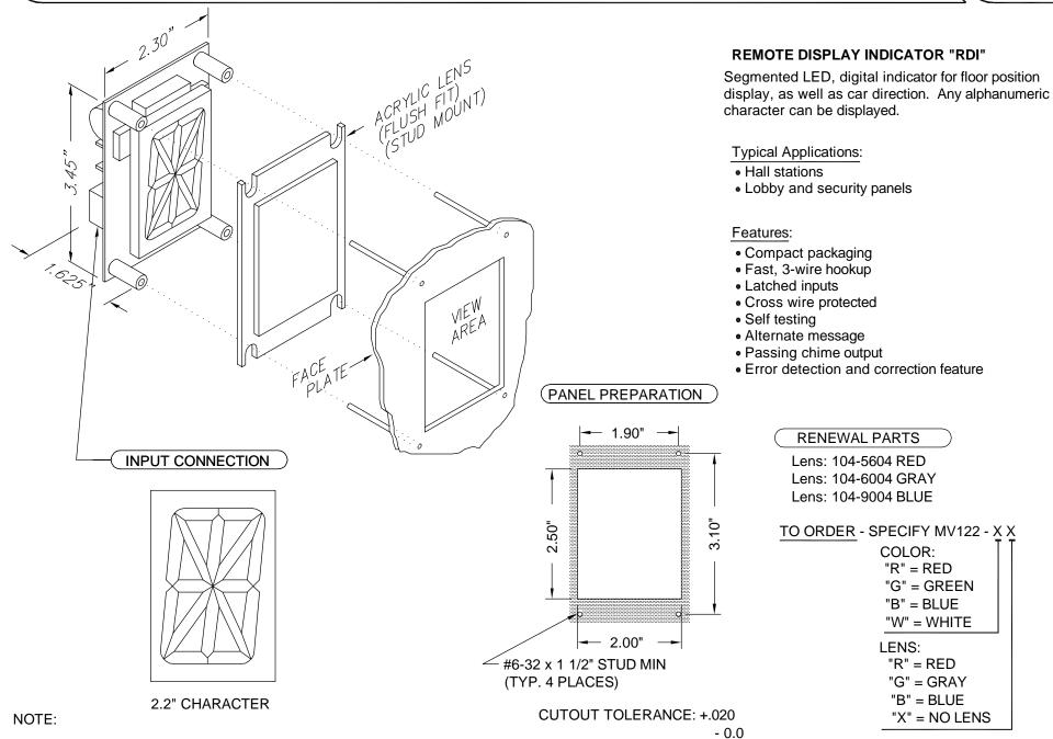
1. This is not a stand alone unit. Must be used in conjunction with a Micro Comm interface.
