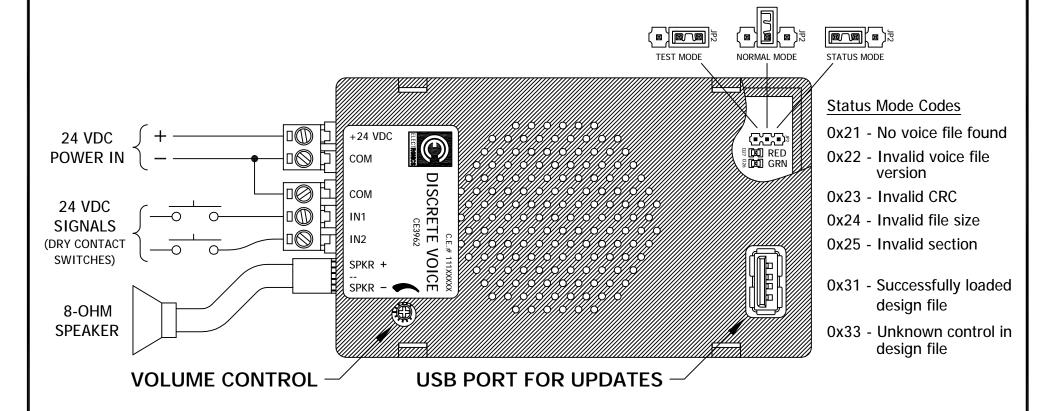
Status Mode LEDs - Using the shunt on JP2 to put the unit in STATUS MODE causes the LEDs to blink a visual code as shown above. For example, '0x24 - Invalid file size' is two RED and four GREEN LED flashes; '0x31 - Successfully loaded design file' is three RED and one GREEN LED flashes.
