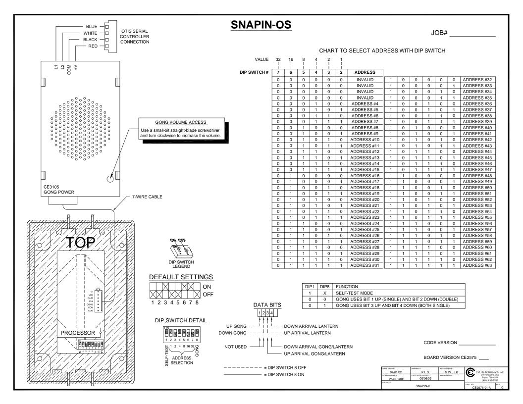
The following Otis data must be furnished at the specified addresses for the Otis Serial Lantern to work properly. The address is selected by setting DIP switches 2-7 as shown on the back of this page. The board reads the address determined by the DIP switch setting. For example, if the DIP switch is set to address 50, the board will read the bits at address 50.
