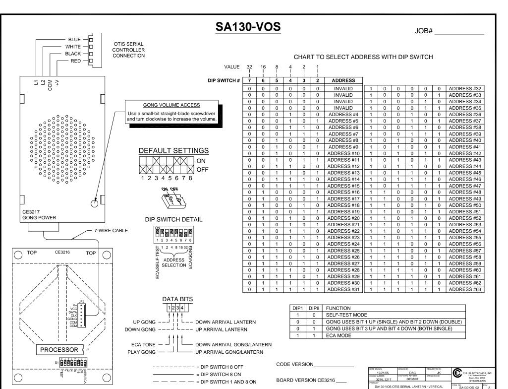
The following Otis data must be furnished at the specified address for the Otis Serial Indicator to work properly. The address is selected by setting DIP switches 2-7 as shown on the back of this page. The board reads the address determined by the DIP switch setting. For example, if the DIP switch is set to address 50, the board will read the bits at address 50.
