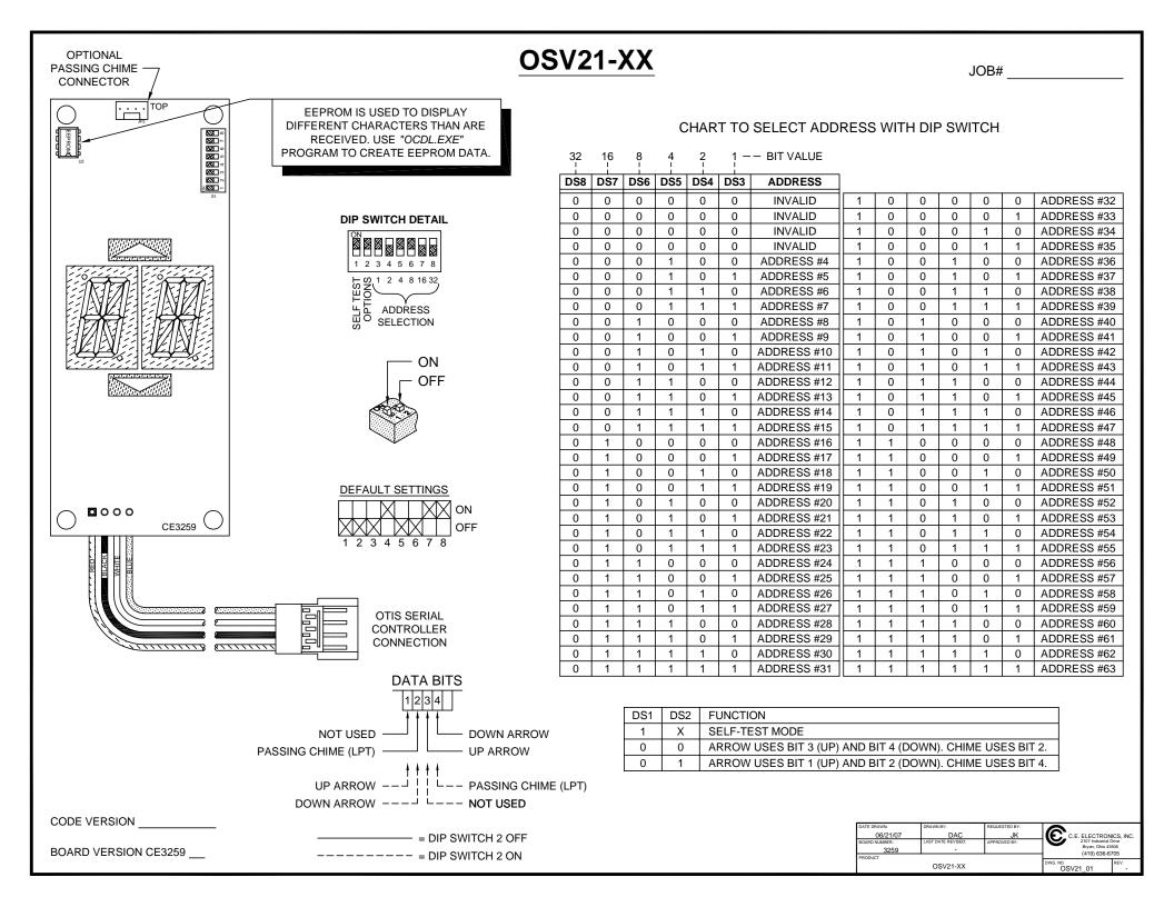
The following Otis data must be furnished at the specified addresses for the Otis Serial Position Indicator to work properly. The address is selected by setting DIP switches 3-8 as shown on the back of this page. The board reads the address determined by the DIP switch setting. For example, if the DIP switch is set to address 50, the board will read the bits at address 50.
