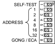
CHART TO SELECT ADDRESS WITH DIP SWITCH
