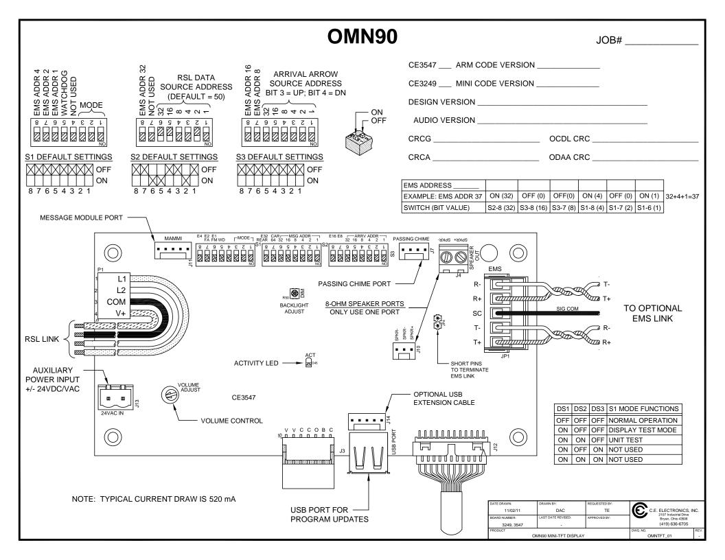
The serial link must contain the following Otis data at the specified addresses for the display to work properly. Select the RSL Data address by setting S2, DIP switches 1-6 using the binary number for the desired address. The board reads five continuous addresses beginning with the address determined by the DIP switch setting. For example, if the DIP switch is set to address 50 (default), the board reads the bits at addresses 50-54.
