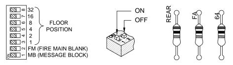
The Micro Comm driver must be programmed to send messages with the level required to activate the features listed below. Level 0 messages will always be displayed, regardless of DIP switch or resistor settings.
