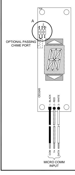
The Micro Comm driver must be programmed to send messages with the level required to activate the features listed below. Level 0 messages will always be displayed, regardless of resistor settings.
