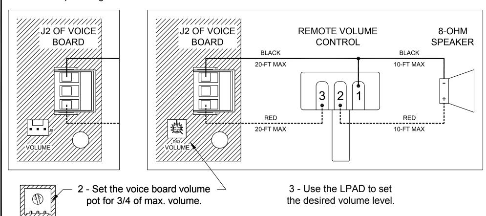
If the LPAD is a replacement for a voice board with an MTA connector instead of a volume pot, connect the LPAD as shown at right and replace the old remote volume pot with the CE3808 board as shown above:
