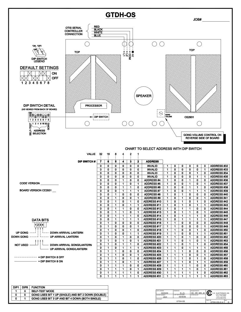
The following Otis data must be furnished at the specified addresses for the Otis Serial Lantern to work properly. The address is selected by setting DIP switches 2-7 as shown on the back of this page. The board reads the address determined by the DIP switch setting. For example, if the DIP switch is set to address 50, the board will read the bits at address 50.
