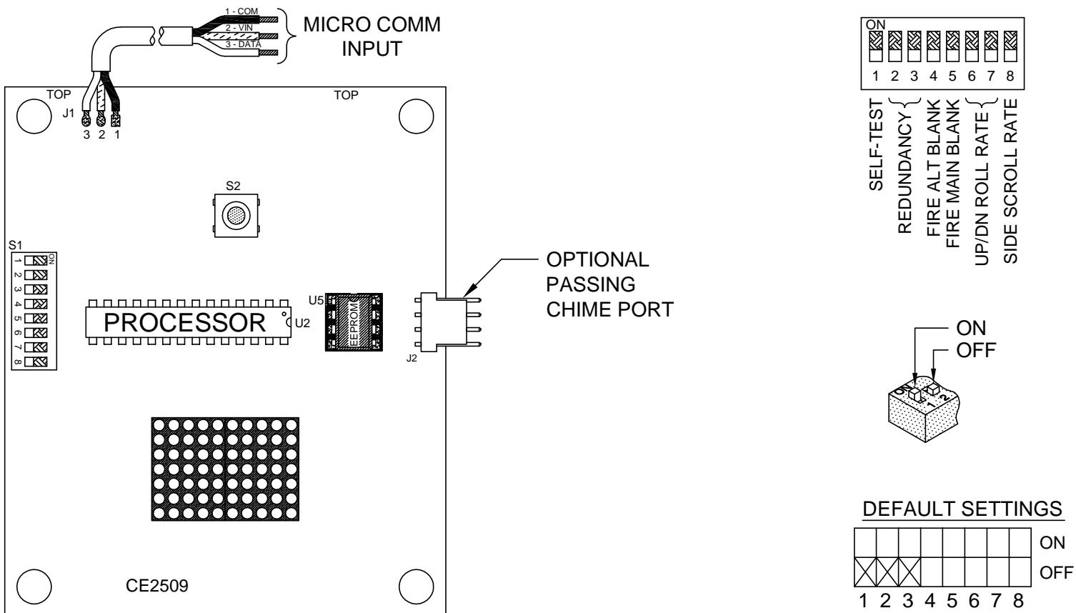
**S2 FLOOR SELECT SWITCH - SETS THE DISPLAY TO SHOW AN ARRIVAL ARROW WHEN THE CAR IS AT A SPECIFIC FLOOR. TO SET THE UNIT FOR ARRIVAL MODE, POSITION THE CAR AT THE DESIRED FLOOR OR TURN ON SELF-TEST. WHEN THE DISPLAY SHOWS THE DESIRED FLOOR, PRESS AND HOLD S2 UNTIL THE FLOOR POSITION CHANGES TO AN ARROW. TO RETURN TO NORMAL OPERATION, PRESS AND HOLD S2 UNTIL THE ARROW CHANGES TO THE FLOOR POSITION.**
