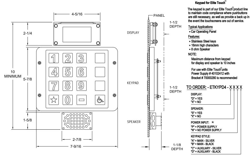
If using CIB-O no Power Supply is required or if 24VDC is available in the COP no Power Supply is required.
