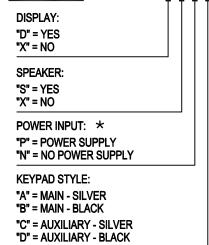
If using CIB-O no Power Supply is required or if 24VDC is avaible in the COP no Power Supply is required.
