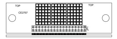
S2 FLOOR SELECT SWITCH - SETS THE DISPLAY TO SHOW AN ARRIVAL ARROW WHEN THE CAR IS AT A SPECIFIC FLOOR. TO SET THE UNIT FOR ARRIVAL MODE, POSITION THE CAR AT THE DESIRED FLOOR OR TURN ON SELF-TEST. WHEN THE DISPLAY SHOWS THE DESIRED FLOOR, PRESS AND HOLD S2 UNTIL THE FLOOR POSITION CHANGES TO AN ARROW. TO RETURN TO NORMAL OPERATION, PRESS AND HOLD S2 UNTIL THE ARROW CHANGES TO THE FLOOR POSITION.
