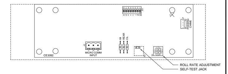
To SELF-TEST display unit, short the two pins on the S2 header and release. NOTE: If S2 is a rotary switch, set it to "F" and back to 0 to self-test.
