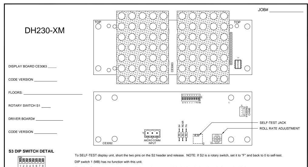
The Micro Comm driver must be programmed to send messages with the level required to activate the features listed below.
