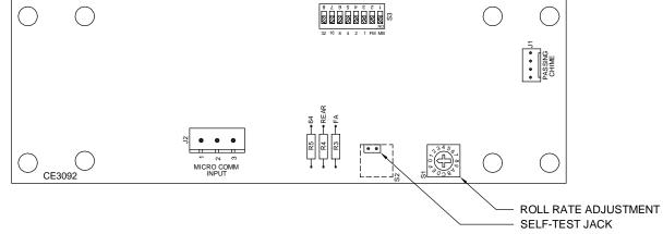
To SELF-TEST display unit, short the two pins on the S2 header and release. NOTE: If S2 is a rotary switch, set it to "F" and back to 0 to self-test.
