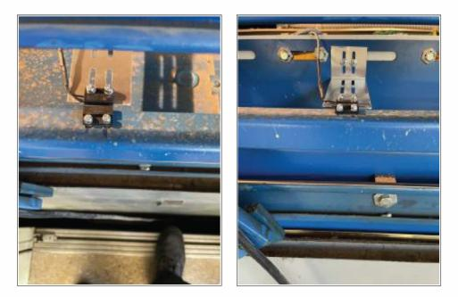
C.E. Electronics recommends installing the DFC Sensor for the **Door Lock Monitoring System** horizontally with a 1/4'' - 3/8'' gap between the magnet and the sensor.
